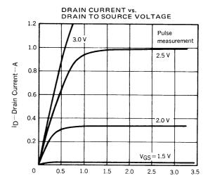
$V_{\mbox{\scriptsize DS}}\!-\!\mbox{\scriptsize Drain to Source Voltage-V}$
