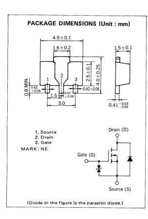
The 2SK1585 is an N-channel vertical type MOS FET which can be driven by 2.5 V power supply.
